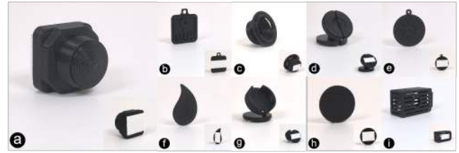
Figure 3: The 3D-printed sensor mockups used in our study. Each mockup includes Velcro on the back, allowing it to be attached to the Velcro strips placed at various locations inside the car interior. The set includes: (a) Camera (b) GPS (c) Microphone (d) Gesture Sensor (e) Light Sensor (f) Humidity Sensor (g) Millimeter-Wave Radar (h) Pressure Sensor (i) Temperature Sensor
