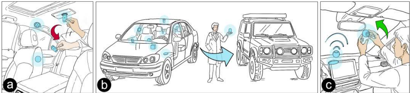
Figure 1: Illustration of the concept of retrofitting car cabins using user-selected sensors. A user can place various types of sensors, such as those monitoring air quality for climate control, gesture input, voice input, or biometric signals like fatigue, at different locations within the cabin to create customized smart cabin experiences. (a) The user can reconfigure the smart cabin experience by relocating or removing sensors. (b) The user can transfer their smart cabin experiences from one car to another. (c) The user installs sensors carried from another vehicle and sets them up in the new car, enabling familiar smart cabin experiences in the new vehicle.
